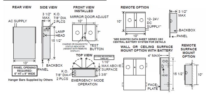
NOTE: THIS DEVICE CONTAINS A MICROPROCESSOR TO CONTROL EMERGENCY LIGHTING. OPERATION CAN BE DISRUPTED BY EMI (ELECTRO- MAGNETIC INTERFERENCE) EMITTED BY CERTAIN TYPES OF HIGH-POWERED EQUIPMENT. DO NOT CONNECT IN THE SAME CIRCUIT OR SHARE NEUTRAL WIRING WITH FREQUENCY-CHANGING DIMMING EQUIPMENT USED WITH HID FIXTURES OR SIMILAR. CONTACT FACTORY FOR MORE INFORMATION.
